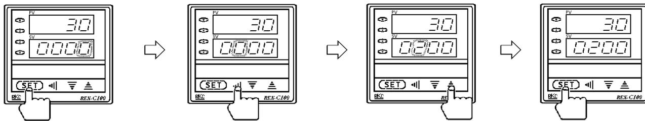
Press the **SET** key to enter the SV setting mode. The digit which lights brightly is settable.
