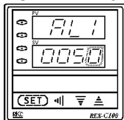
Press the **SET** key for more than 5 sec. to set controller to the parameter setting mode.
